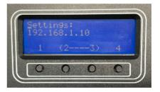
appearing LED number buttons on the Broadcast Panel and press SAVE Server IP.
