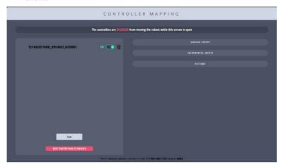
13. If you select the controller, it appears as green meaning that the appearing controls on the right of the page are those for the selected joystick and can be configured.
