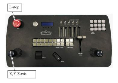
Network Broadcast Panel with Dual Joystick has an additional joystick that can be configured to use 3 additional axis on the robot in Flair. The other controls and button work exactly as the single joystick version. For details refer to *Controls: Network Broadcast Panel* on page 11.
