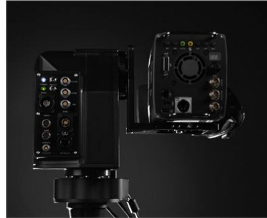
Integrated I/O and optional slip rings allow for easy field deployment and simplified camera cabling. Lens control of digital and manual lenses is also built-in, further reducing cable runs. Fibre and wireless interfaces are available to extend the AFC and camera RCU operating distances.
