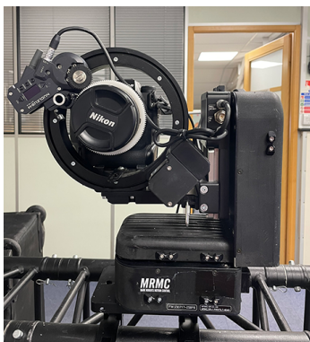
SR-1 head Overslung mounted on a truss using the mounting plate
