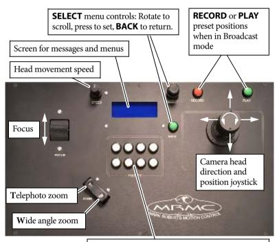
Eight **PRESETS** for recording and playing back static camera positions when in Broadcast mode, and playing back moves when in Film mode.
