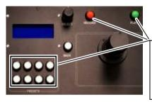
Once in Broadcast mode you record, use, and modify presets by using the **RECORD**, **PLAY**, and **PRESETS** buttons. No menu is required.
