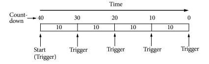
Note that because the controller takes frames at both the start and end of the move, it actually takes a total of FRAMES+1 frames, so 5 total frames in the above FRAMES: 4 example. This makes it easy to calculate the total time as FRAMES  $\times$  FRAME TIME.
