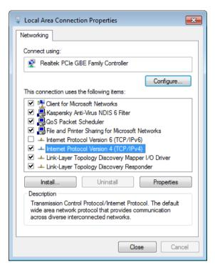
5. In the Local Area Connection Properties pop-up that appears, on the Networking tab, switch on and select Internet Protocol Version 4 (TCP/IPv4) then click on Properties to see the IP address settings. For example:
