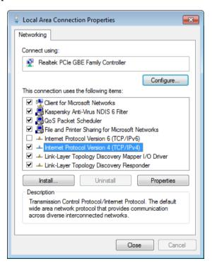
5. In the Local Area Connection Properties pop-up, **Networking** tab, switch on and select **Internet Protocol Version 4 (TCP/IPv4)** then click on **Properties** to see the IP address settings.
