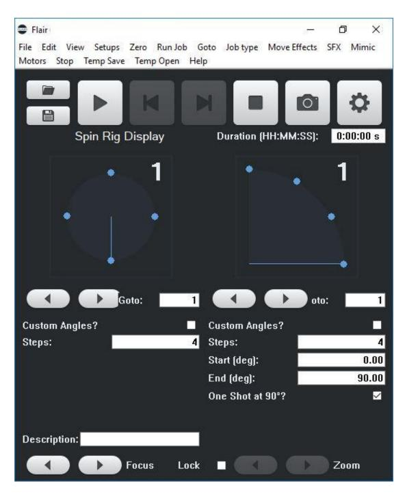
The basic theory of the spin rig is that a number of horizontal rotational angles and vertical elevation angles can be defined and the item is then photographed from each of these positions, going in sequence rotationally or vertically. This will result in a complete visual recording of the item from all angles.
