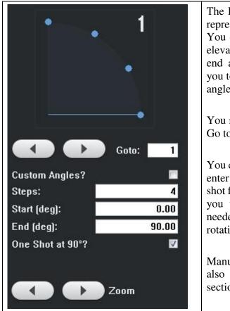
The Elevation controls show a graphic representation of the elevation points. You can set the number of steps in the elevation motion as well as the start and end angles. The arrow controls allow you to move the spin rig to the different angles.
