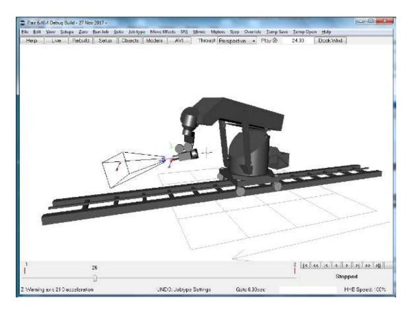
The display is a 3D view that allows you to view the rig through a Perspective or Orthogonal camera as well as being able to view through the camera mounted on the rig. Many of the rig designs that are used with Flair are supported and carefully picking your kinematics model will assist in making sure that the rig is properly displayed.
