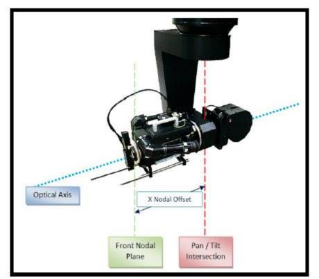
26. Enter in the Z and Y Nodal Offsets as measured from the intersection of the pan and tilt axes. The Y offset is positive going to the left (looking from the back of the
