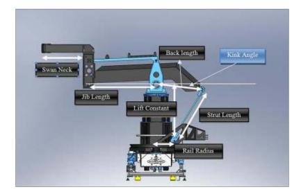
**Lift Constant:** This is the height of the lift pivot above the rotate ring when the arm is level. This is the required position for the lift zero. It is measured vertically from the arm pivot to the lower swing strut pivot.
