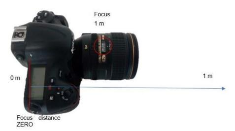
18. If your measure hook (the point that you will usually measure from) is not at the film plane, then enter the distance from the film plane to your measure hook measured in metres into the Measure Offset in the Lens Setup display. SAVE and APPLY the setup. If the measure offset is not 0 the focus distance in Flair will NOT match the focus value on the lens.
