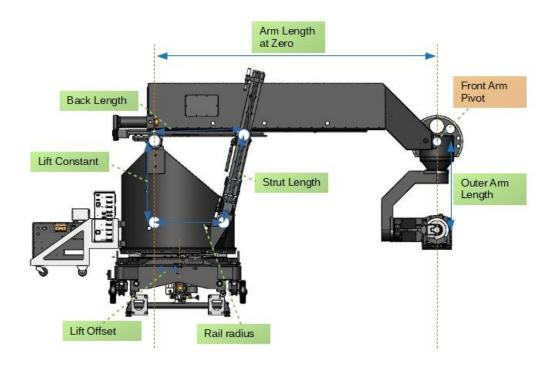
Lift Constant: This is the height of the arm pivot above the lower lift pivot.
