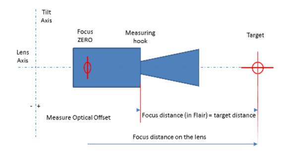
29. Measure Normal Offset is the distance from the measure hook to the Optical Axis measured perpendicular (normal) to the Optical Axis.
