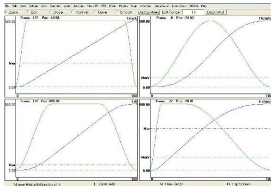
Diagram shows position and velocity graphs for the same two waypoints but with different fairings. Track – 10% fairings. Lift - 30% fairings. Rotate – 50% fairings. Extend – 10% up fairing, 70% down fairing.
