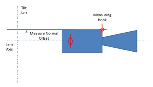
Measure Normal Offset give a very accurate positioning of the target when in target tracking, which is required for scaling and other advanced features and it is recommended that for normal use you ignore this offset and set it to 0.0. Often when close up the distance to the target is measured parallel to the optical axis and in that case this offset is irrelevant.
