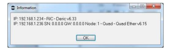
Here we can see the addresses of the responding nodes, the first at 192.168.1.234 is the RIC board (usually referred to as an RT12 or RT14) and it is running the program Deric v6.33. The attached axis node is Node 1, has the address 192.168.1.236 has no Subnet (SN) or Gateway (GW) assigned and is a Quad Board running Quat Ether v6.15. (Gateway and Subnet are not advanced configuration and are not used with standard Network Direct.)
