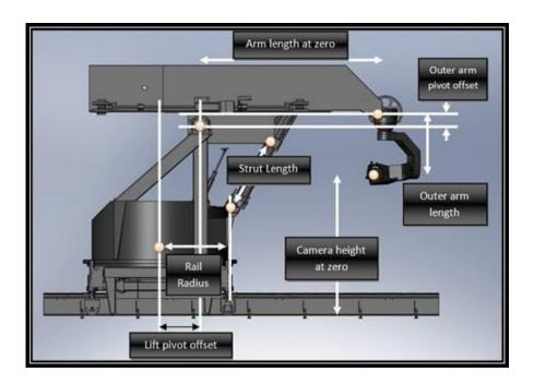
**Outer Arm length:** This is the length of the outer arm, also called the Angle or Pitch. The distance is from the axis about which it rotates to the tilt axis. This value may be used to assist in drawing the head in the Rig Model display.
