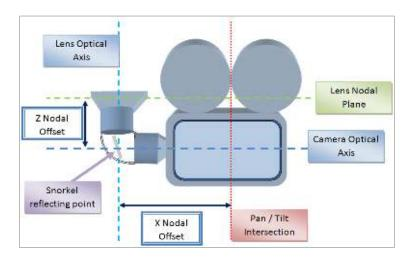
**Notes on Y&Z Nodal Offsets:** You can use Y&Z Nodal Offsets with a rig that has a tilting pan axis (e.g.: Cyclops, Milo, Overhead etc) but these offsets will ONLY work when you are in Keep Horizon Level or Keep Horizon Relative. If you are not in this mode, or if this mode has turned itself off, then the move will not necessarily match the programmed move. This is particularly true when you are importing XYZ data.
