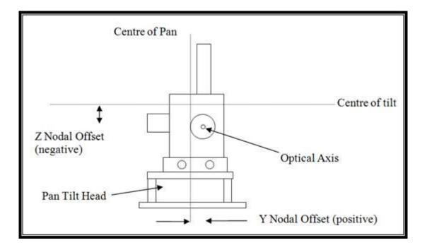
**Z Nodal Offset:** This is the vertical distance from the centre of the tilt axis and the front nodal point of the lens. Again this distance is usually 0.0. For a snorkel lens this is from the front nodal point of the lens to the Snorkel Reflecting Point. The Z Offset is measured positive going up.
