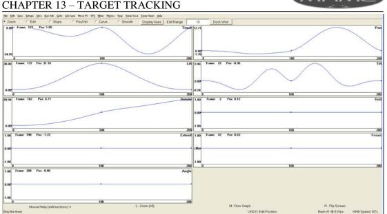
Adding points on the Cartesian Graphic display will add a blank line with a waypoint on it for only that axis. As covered above, this is not recommended practice. Nor is deleting waypoints for one Cartesian axis.
