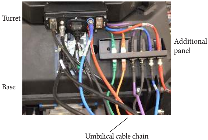
Picture of umbilical - base - turret connections:
