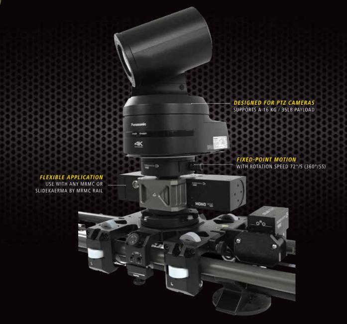
The PTZ Monohead enhances the horizontal axis motin for PTZ camera productions. The head provides fixed-point tracking for remote heads. Since PTZ cameras cannot perform this precise motion, the PTZ Monohead adds another panorama axis that replaces the horizontal movement by rotating the whole unit. Thanks to this simple trick, you can control the horizontal rotation of the kit, keeping all other benefits of your PTZ system.
