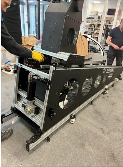
5. To attach the drag chain, locate the spacer on the lift motor and loosen the 2 x countersunk screws on the plate on the end of the
