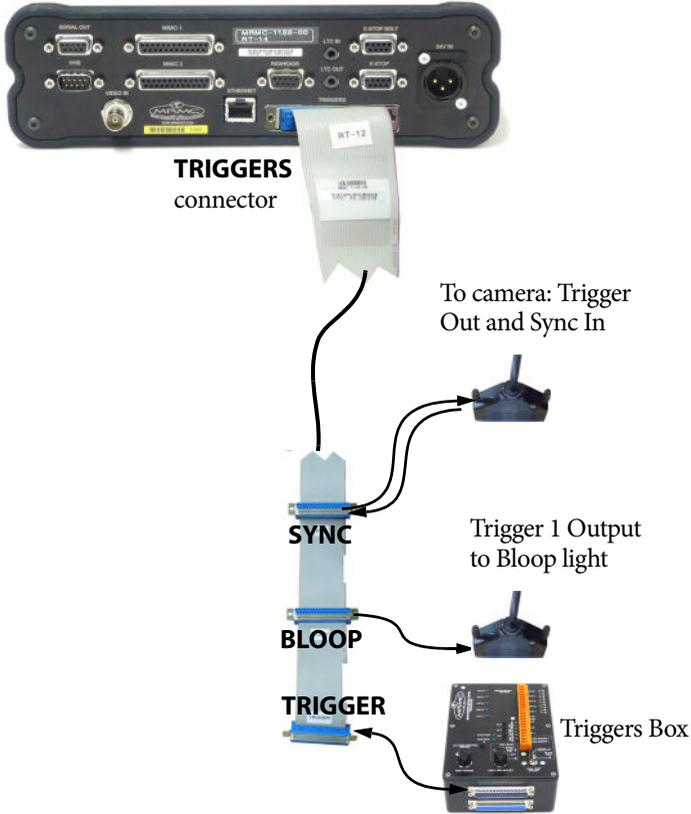
The External Camera Trigger Out and Sync In are directly connected to the camera.
