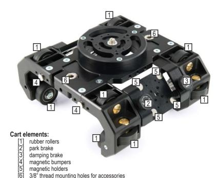
The ATLAS MODULAR slider's cart is equipped in 12 rollers, made of specially assorted hardened rubber [1]. Thanks to the proper location of the rollers the slider can move in a horizontal, inverse, vertical and slanted position.
