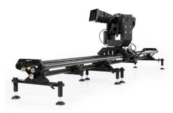
Connection of the ATLAS MODULAR slider's drive and the SLIDEKAMERA controlled head (X HEAD or BULL HEAD) allows creating a full motion control system. Thanks to the combination of the slider's drive and the head the user gets an integrated system, which can be controlled with a single controller or the Slideye PRO application for mobile devices.
