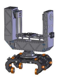
In order to remove the head safely (e.g. for transport) it is enough to loosen the clamp screw and pull out the head together with the plate out of the adapter's base.
