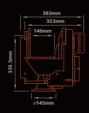
SFH-50 with Tilt Support & Pan Spacer
