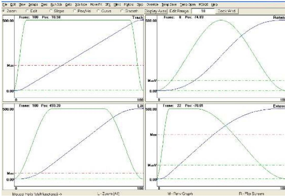
*Diagram shows position and velocity graphs for the same two waypoints but with different fairings. Track – 10% fairings. Lift - 30% fairings. Rotate – 50% fairings. Extend – 10% up fairing, 70% down fairing.*
