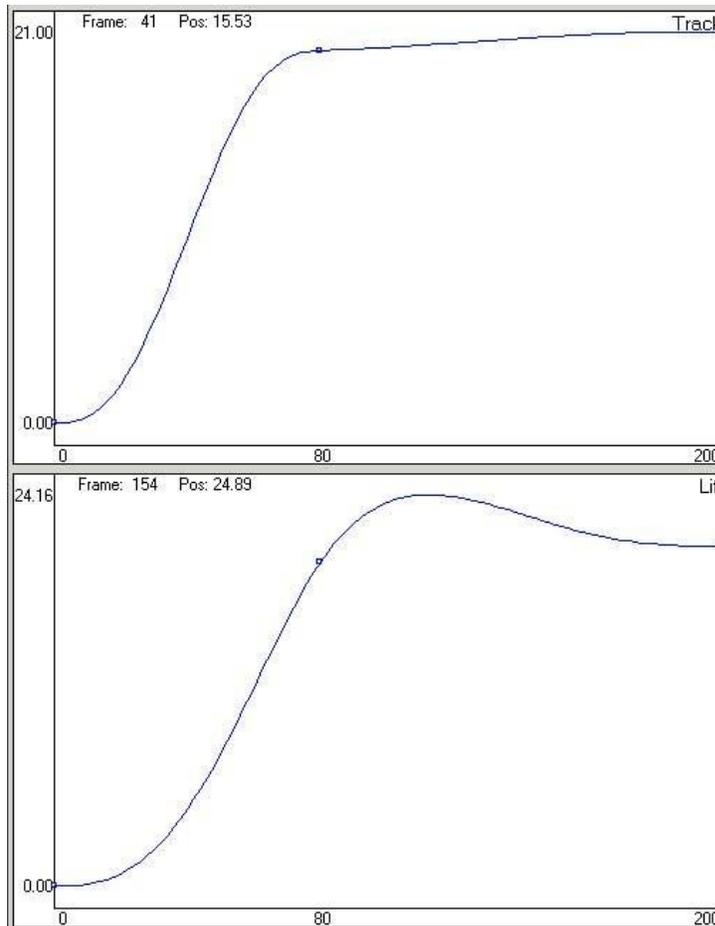
Here is an example of a curve which reverses, and one which has been handled. The movement and timings are the same on the 2 axes, but the lift clearly exceeds its end position during the move, but has a nice smooth curve. The Track has had curve reversal handled and does not exceed its end position, but it is 2 connected moves, and is not as smooth as the lift's motion.
