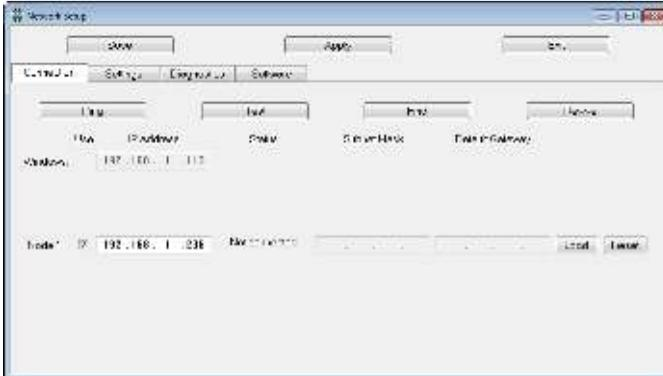
The Network Setup window, Connection tab, lists the Nodes (head connections) that Flair is looking for, as defined in the NetworkDirect.ini file. Any changes that you make and **Save** in the Network Setup window are saved in the NetworkDirect.ini file. You can also edit this file by using the menu option **Help > View Network .ini File**. If Flair cannot find the head on the network at the IP address shown then the node's status is **Not connected**.
