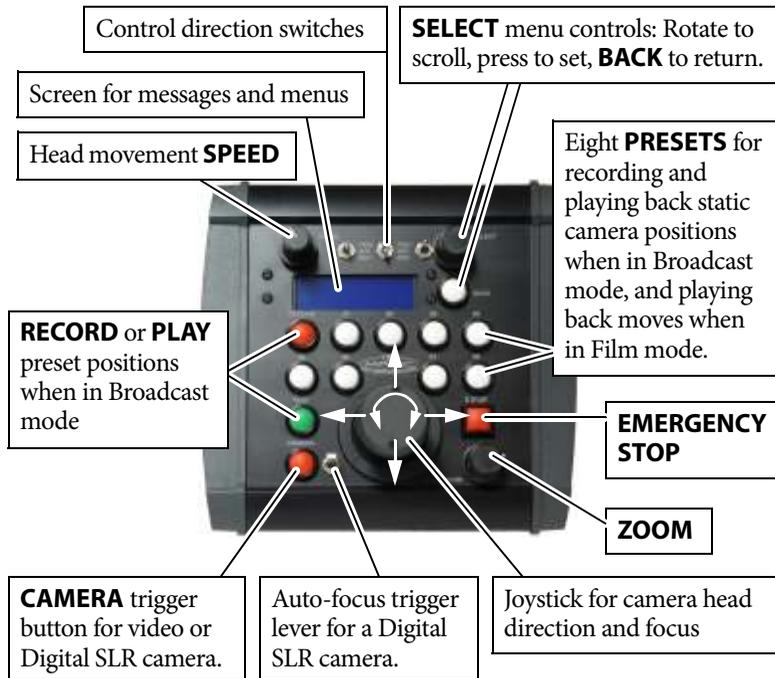
On the Mini MSA, the rotation of the joystick is typically assigned to the lens focus.
