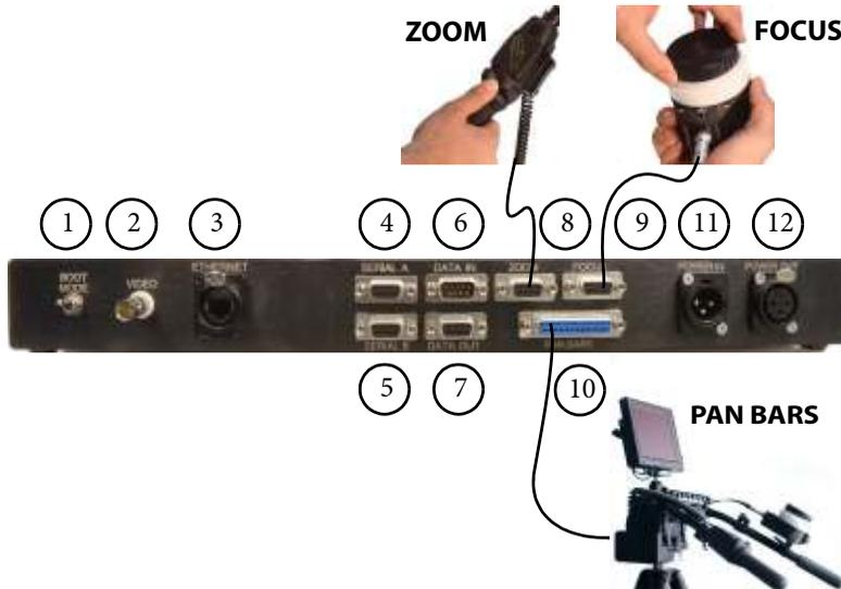
1. **BOOT MODE** switch. The mode in which to start up. One of:
