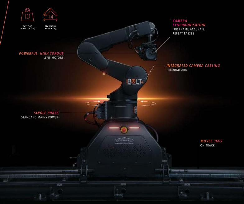
Bolt Jr+ is a compact, lighter weight high-speed camera robot with a longer reach than the Bolt Jr. The agile, smaller rig also comes with an increased camera payload (10kg) and is an ideal solution for smaller spaces or location work.
