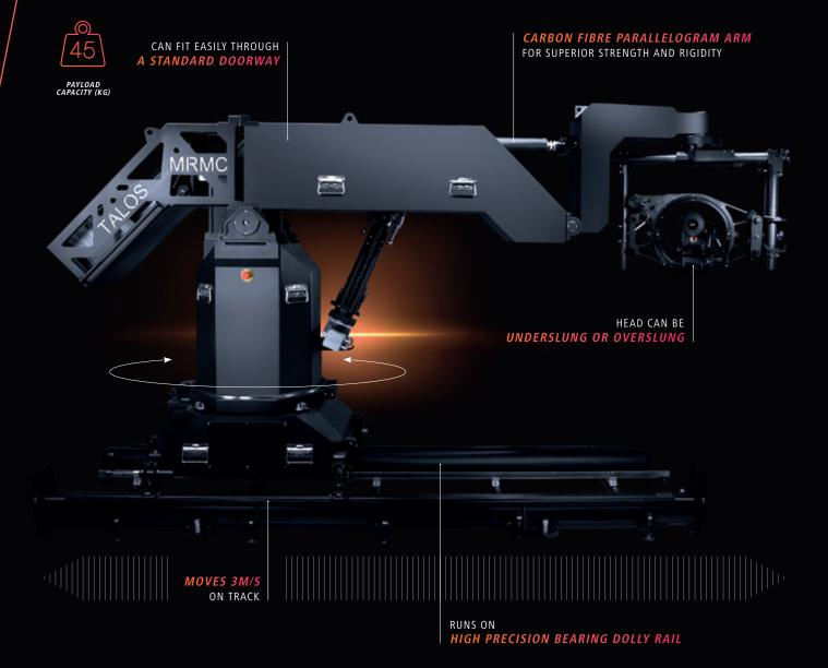
The Talos is a medium sized rig designed for easy, portable motion control – making it ideal for location work. Half the weight of the larger Milo rig, the Talos still offers a wide operating envelope, making it a good alternative for shoots where space or transport is a factor.
