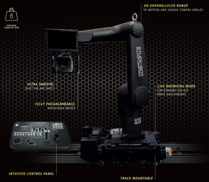
The StudioBot is a 9-axis robotics system offering a superior creative range to traditional dolly systems. With a smaller physical footprint than the larger XL system, the StudioBot is ideal for small-scale studios. Offering all the benefits of integrating with studio automation and 3d graphics systems, the StudioBot creates a vast range of programmable and repeatable shots for studio environments.
