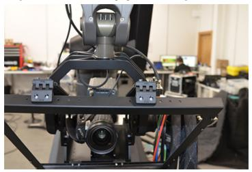
3. Detach the camera plate from the camera platform. Mount the camera on the long side of the camera plate using 2 x thumb screws.
