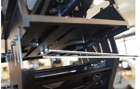
Screw the camera plate to the camera platform
