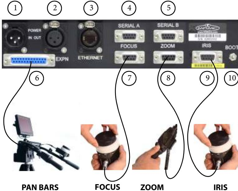
1. **POWER IN** connector. The Joystick Controller requires a 3-pin, 24 Volt DC power supply. For pin-out information see *Power In connector* on page 123.
