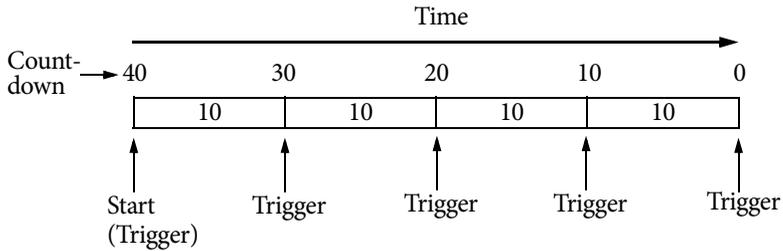
Note that because the controller takes frames at both the start and end of the move, it actually takes a total of **FRAMES+1** frames, so 5 total frames in the above **FRAMES: 4** example. This makes it easy to calculate the total time as **FRAMES × FRAME TIME**.
