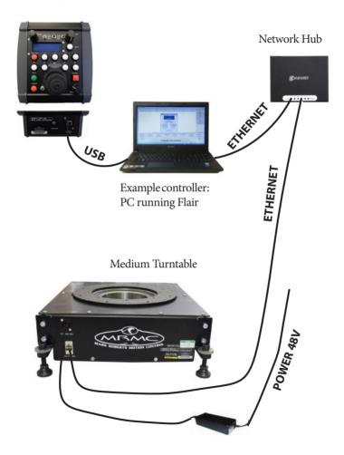
The diagram shows a typical application. Attach the power cables last. The controller can be any MRMC controller such as a PC running Flair Motion Control Software or one of the MSA-based controllers such the Large Flat Panel (LFP), MSA-21 Handwheels, Joystick Controller, or Mini
