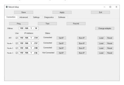
The Network Setup window, Connection tab, lists the Nodes (board and head connections) that Flair is looking for, as defined in the NetworkDirect.ini file. Any changes that you make and **Save** in the Network Setup window are saved in the NetworkDirect.ini file. You can also edit this file by using the menu option **Help** > **View**
