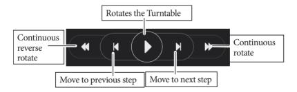
The Continuous Rotate buttons can be used for product video shoot. When a move is playing, this bar replaces the Play button with the Stop button that can be used to stop the Turntable at any point.
