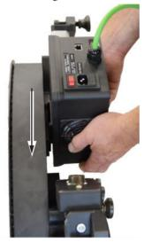
2. Use an allen key to tighten the grub screw to secure the control box to the Large Turntable.
