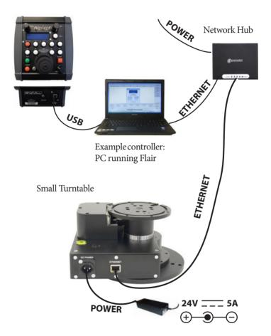
The diagram shows a typical application. Attach the power cables last. After this, to add the turntable in Flair, refer to *Adding Ethernet Turntables in Flair* on page 15. The controller can be any MRMC controller such as a PC running Flair Motion Control Software or one of the MSA-based controllers such the Large Flat Panel (LFP), MSA-20 Handwheels, Joystick Controller, or Mini MSA.
