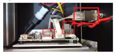
3. With the new pane, plug the stepper motor into the 7 way plug then plug the other side onto the PCB. There is only one place it will fit.
