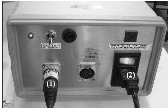
Figure 5. Power Supply Unit with connections.
