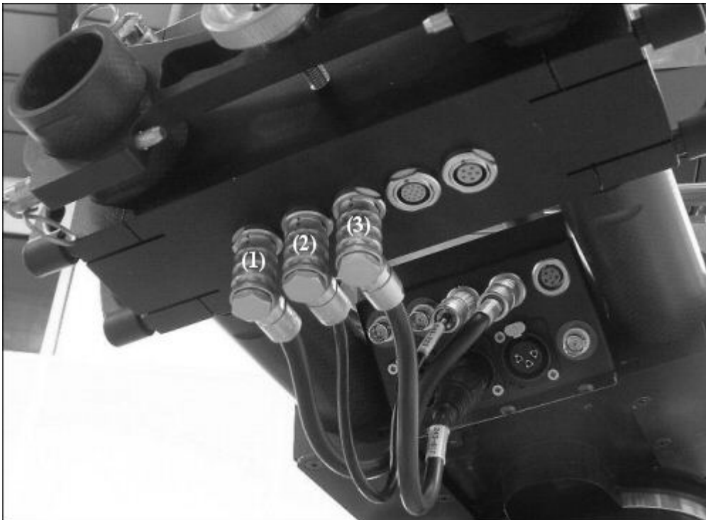
Figure 4. Ulti-Head Slip-Ring lower panel and Ulti-Head Elbow lower panel with (Standalone) connections.
