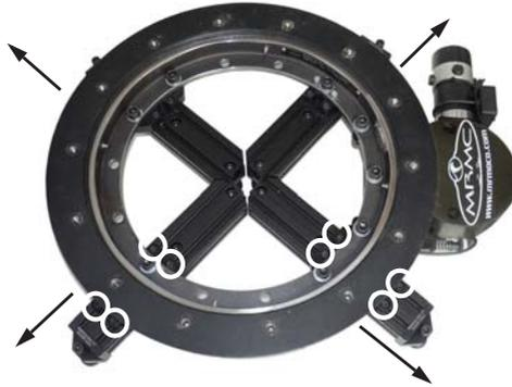
1. Loosen the four screws on each leg to adjust the leg for supporting larger objects on the turntable.
