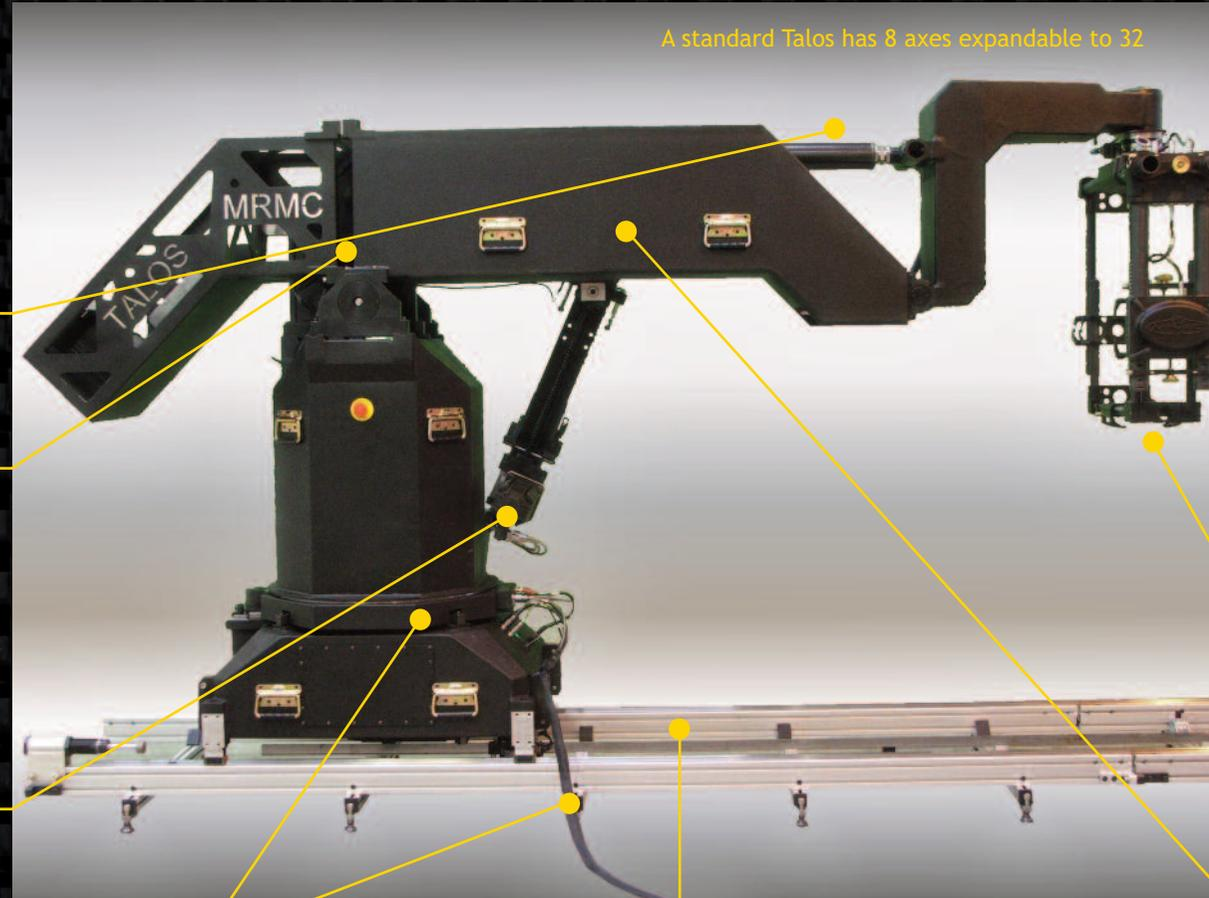
The Talos utilises the popular Ulti-Head which has the ability and additional benefit to be removed for use as a stand alone MOCO or Remote head.
