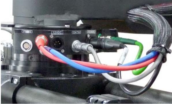
Attach the cables to the head and camera. Here is an example of the cables attached to the Ulti-head.
