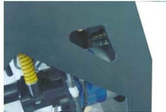
3. Retract the overcenter lock mesh bracket and secure it by inserting an allen key into the slot.
