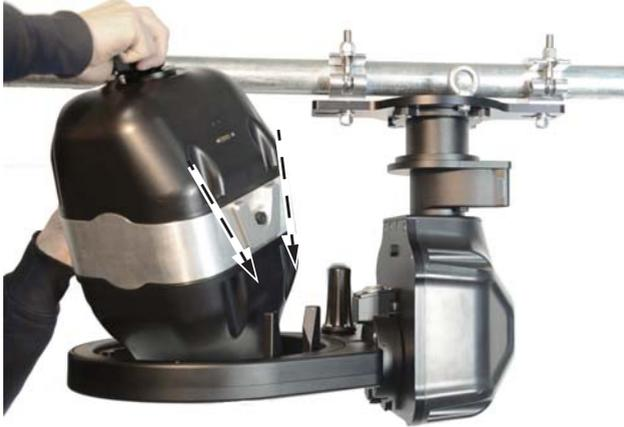
5. Tighten the three screws on roll ring to secure the Pod into the head.
