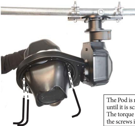
The Pod is not secure until it is screwed in. The torque setting of the screws is 11.2Nm.
