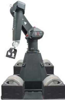
**Bolt On Pedestal** has a stationary base which you either hold down with weights or, for more permanent installations, attach to the floor.
