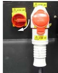
The Bolt power-up sequence takes about three minutes. When it has completed, the Stäubli CS8 shows an “A” on its display.
