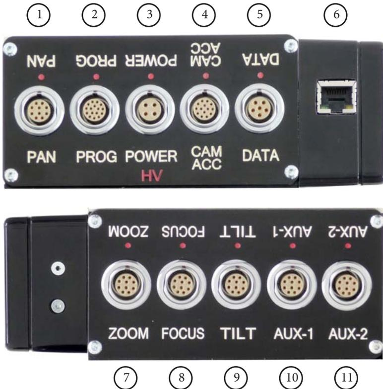
1. **PAN** connector for the Pan servo motor on a head. For pin-out information see *Servo motor connector* on page 38.
