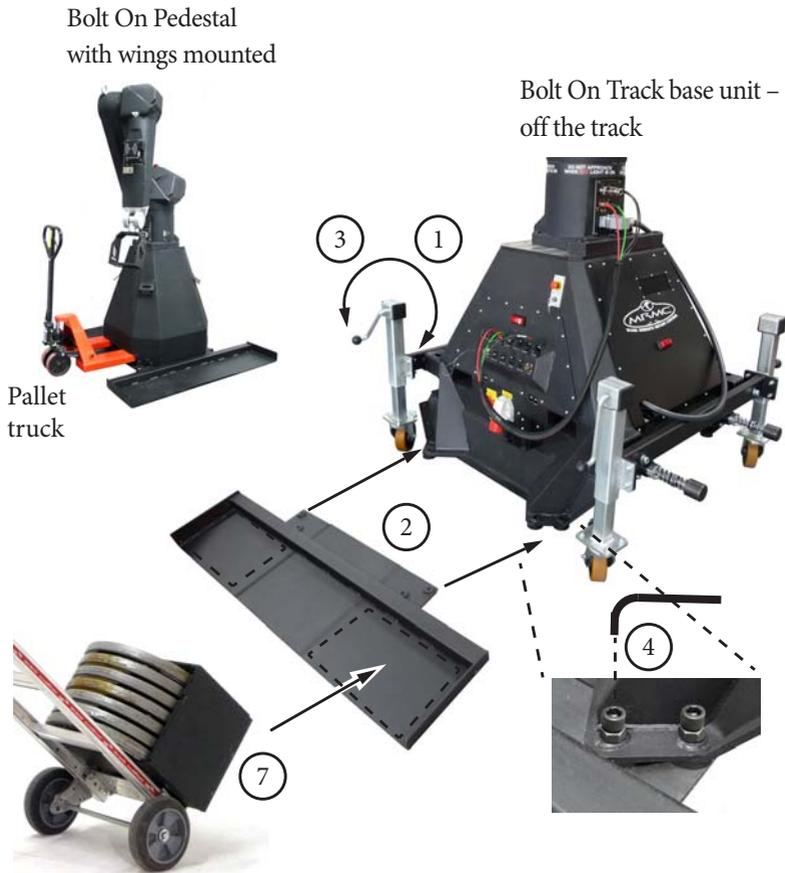
1. Use the wheels (for Bolt On Track) or a pallet truck (for Bolt On Pedestal) to lift Bolt high enough to go over the wings (about 4 cm).
