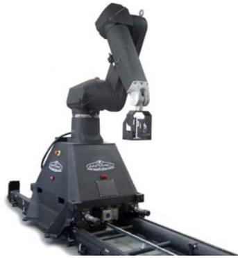
**Bolt On Track** has a base designed for moving along Precision Track. It has removable trolley wheels for moving between sets, and can also be held down with weights at temporary locations.
