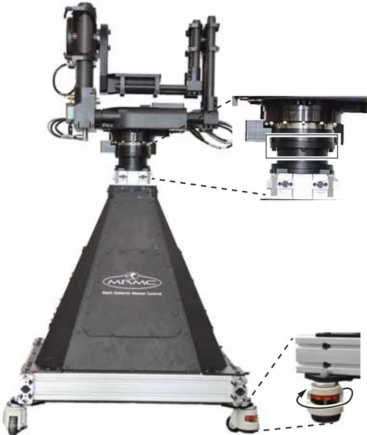
2. Wheel the rig to the desired spot and secure in position by tightening the grub screws in the four castors.
