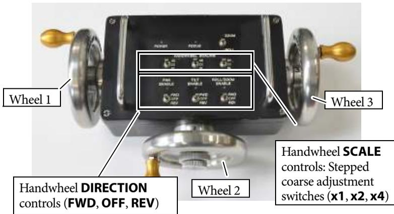
On the Mimic Handwheels, two of the handwheels are typically assigned to the Pan and Tilt head axes, and the third handwheel is typically assigned to Roll or Zoom, although you can change the assignments in Flair if you want.
