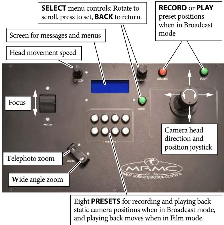
On the LFP the rotation of the joystick is typically assigned to Roll or lens focus, if such a facility is available.
