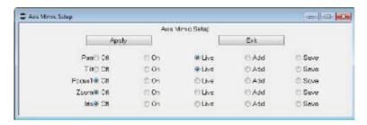
13. Specify **Live** for the axes that you have assigned the Pan Bars to, then **Apply**. After you have tested the mimic operation you can use other settings; see the Flair manual for details.
