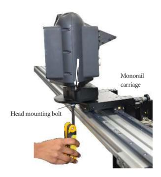
When mounting the head, make sure you line up the key (on the carriage) with the slot in the head.
