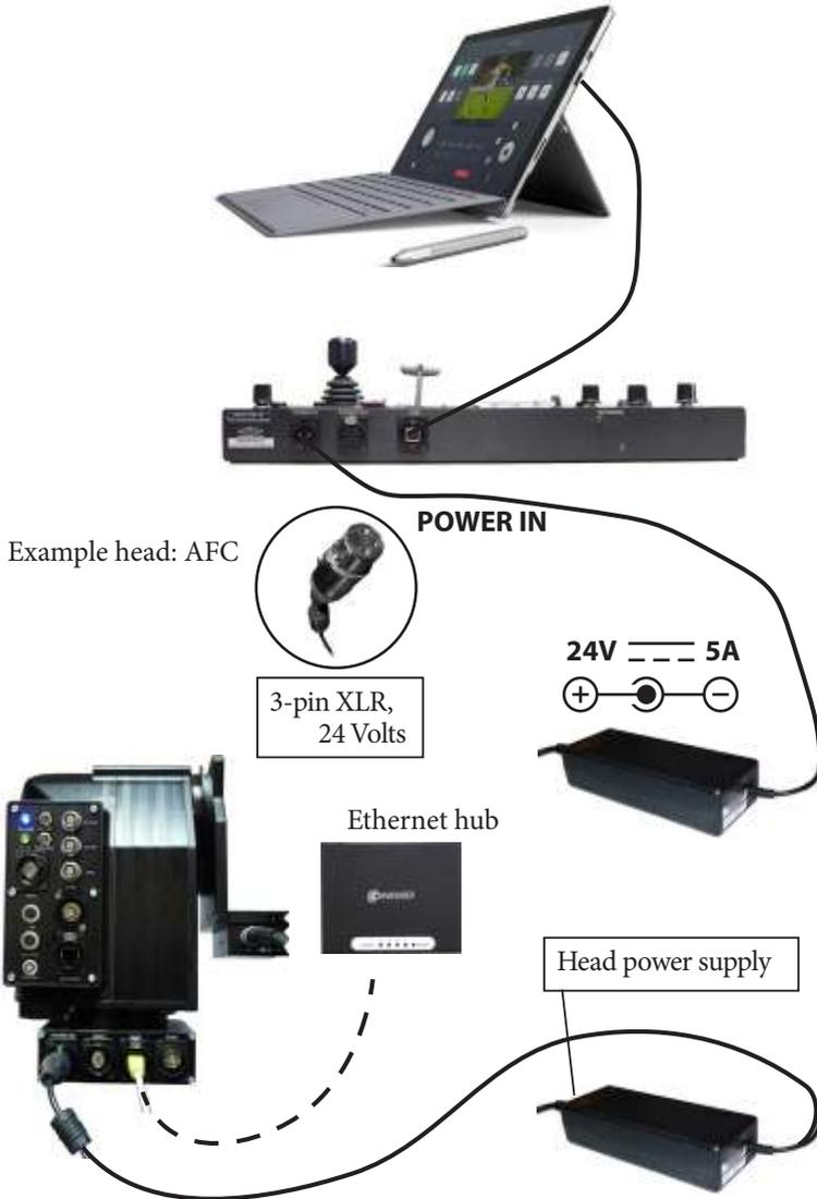
1. Connect the head to the PC running MHC using Ethernet.
