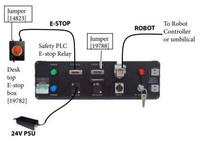
Bypassing RT-14 will make the safety circuit IGNORE the software E-stop and the HHB E-stop that is plugged into RT-14. This should be used only temporarily and the key put back in vertical position soon after.
