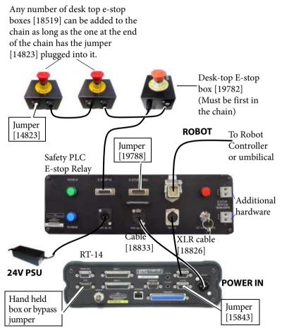
Only one main E-stop box [19782] is used per safety relay box, which is plugged to the **E-stop In** connector.
