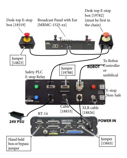
You can even use Broadcast Panel with Ear [MRMC-1525-xx] for robot operation and emergency stops as well. Again any number of Broadcast Panel with Ear and desk top E-stop boxes [18519]'s can be added to the chain in any order as long as the unit at the end of the chain has jumper [14823] plugged into it.
