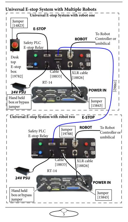
Any number of Universal E-stop Systems can be added to the chain as long as the one at the beginning of the chain has the Desk top E-stop box plugged into **E-Stop In** and the one at the end of the chain has a jumper plugged into **E-stop Thru** connector.
