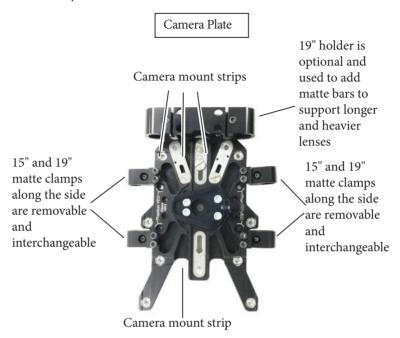
2. Mount the camera on the Camera Plate by aligning your camera with the slots in the camera mount strips and then tightening the UNC camera screws. There are both 1/4" and 3/8" camera mount strips which can be swapped to fit most cameras
