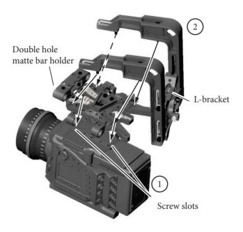
2. Mount the L-bracket on the camera plate such that the double hole matte bar holder is under the ends of the L-bracket. Tighten the 4xM6 screws and washers.
