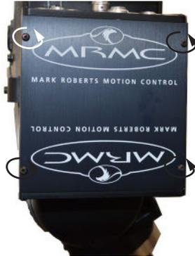
2. Replacing the 4 x screws with longer ones, mount the Focus assist box by attaching it to the Ulti box.
