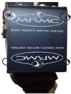
2. Replacing the 4 x screws with longer ones, mount the Focus assist box by attaching it to the Ulti box.
