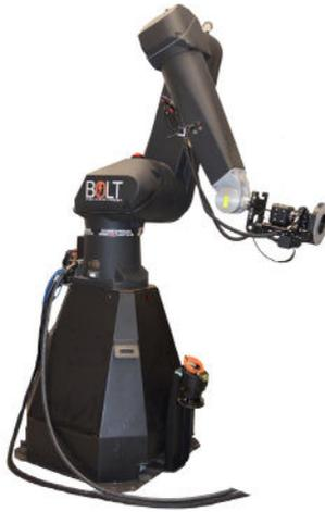
**Showbolt** has a stationary base which you either hold down with weights or, for more permanent installations, attach to the floor.
