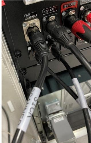
6. In order for the programme to detect the device, it might need to be power cycled by unplugging the grey ‘scanner’ cable from the E-Stop connector box and then re connecting it again after a few seconds.
