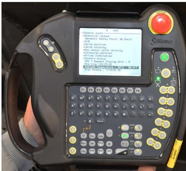
5. Remember to replace the Teach Pendant with the bypass plug after you have completed the procedure.
