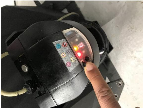
Remove any objects placed in the safe zone area. The light on the sick sensor must be green for the E-stop to be released again.
