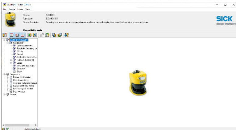
16. To be able to change the “scan window” that is seen by the system and to set a “No Go” zone, you will need to adjust the **FIELD SETTINGS**.
