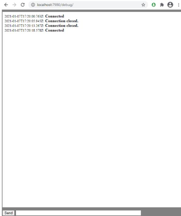
At the top (big white) box you will see the messages from the server and at the bottom part you can send instructions (commands) to the server by typing in the command to the input box and after that pressing the send button.
