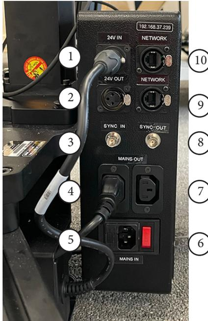
1. **24V IN** input connector for power to the PTA-2 head. This usually connects to the SLH/TRH or Dual Rail **24V OUT** connector via the umbilical. For connector pin-out, refer to *24V In connector* on page 11.
