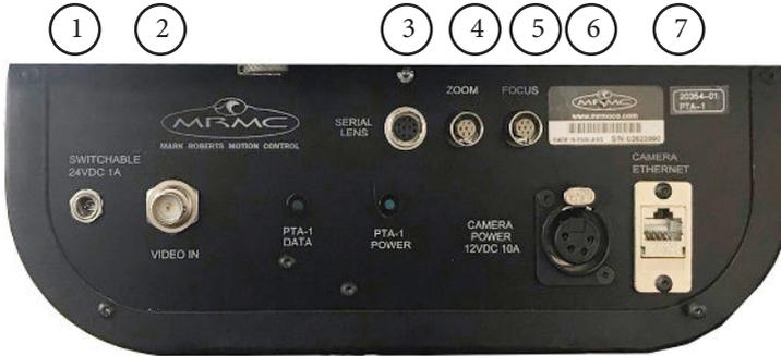
1. **SWITCHABLE 24VDC 1A** connector is the 24V DC outlet for powering a camera or HDMI/SDI signal converter. Centre positive.
