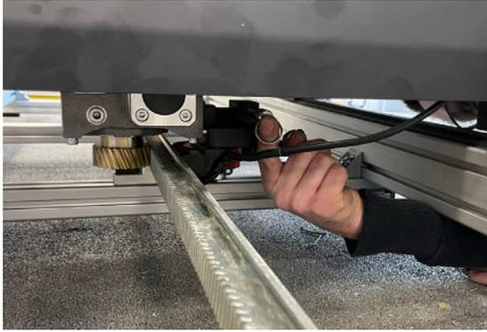
5. Hand-tighten the star knob so that the rubber wheel presses against the smooth side of the rack until you start feeling pressure on the red wheel. You must still be able to turn it easily by hand. This holds the track motor gear firmly against toothed side of the rack.
