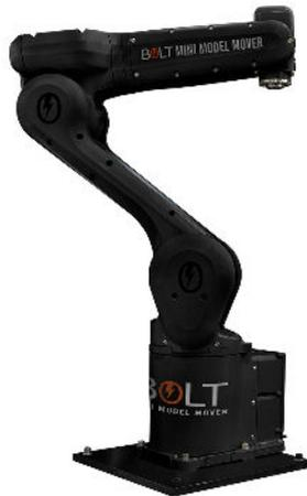
**Bolt Mini Model Mover's** base plate can be attached to a mount of your choice such as wood top using the base clamps.
