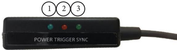
1. **POWER** LED illuminates when the Universal Camera Sync box is connected to the Camera Accessories port on the robot.
