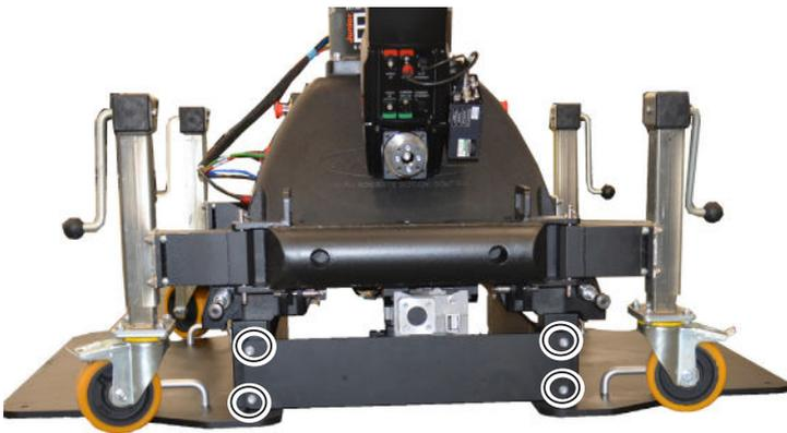
7. Similarly, mount the plate side support on the opposite side. Then, place the weight each plate add 140kg of weights on each weight bucket.
