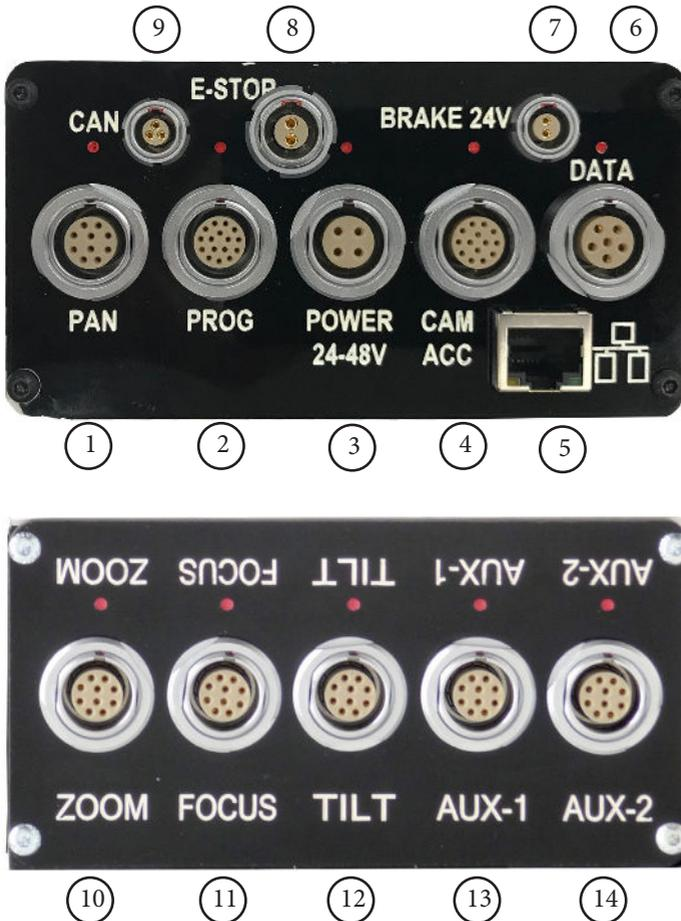
1. **PAN** connector for the Pan servo motor on a head. For pin-out information see *Servo motor connector* on page 46.
