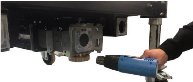
4. Once the pinion is sufficiently expanded, using heat-proof gloves, try removing the pinion; again without using much pressure.
