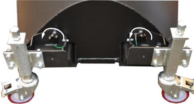
5. Attach the bridges with two weight plates on one side using the 4xM10 screws that attach to the weight plates and 2xM10 screws that attach to the pedestal base.
