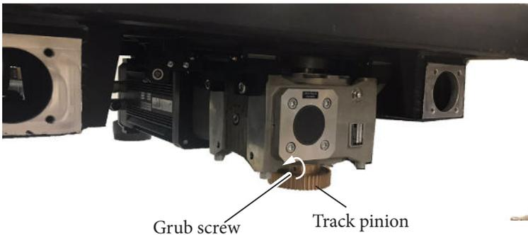
3. You should now be able to release without applying pressure. If it is not released easily, use Flair to run the track motor at a slow speed,
