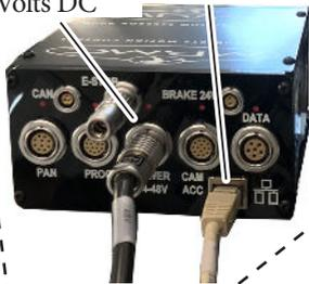
Ulti-box, which provides various connectors for camera and lens controls. For details see *Ulti-box connector summary* on page 43.
