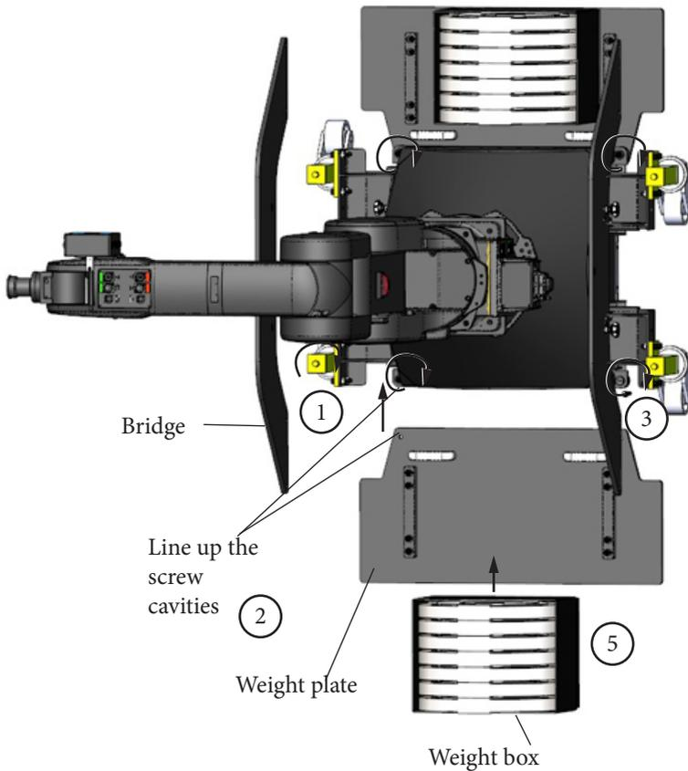
1. Use the jack screws on the castor wheels to lift the base high enough to insert each of the weight plates on either side of the Bolt Jr+ Base lining up the screw cavities.
