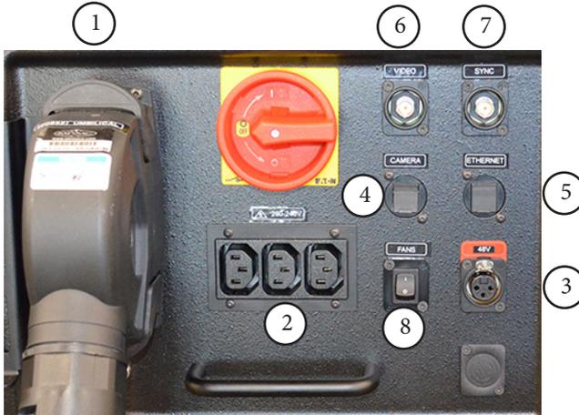
1. **UMBILICAL IN** connector is the main connector that provides 240V single phase power for the controller unit, robot arm and other units on the arm such as Ulti-box and camera. It also includes other connectors for E-stop, video out, sync out, Ulti power and Ulti Ethernet.
