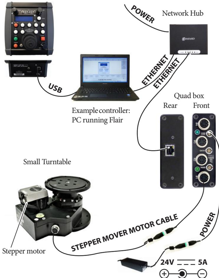
The diagram shows a typical application. Attach the power cables last.
