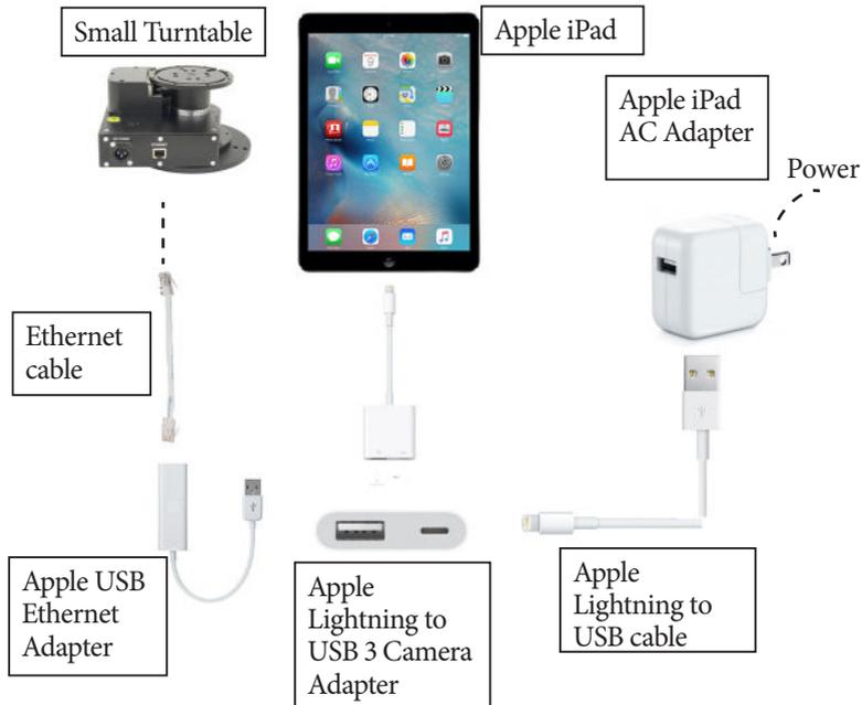
1. Connect the Lightning input on the Apple USB3 Camera Adapter with the Apple Lightning to USB cable.
