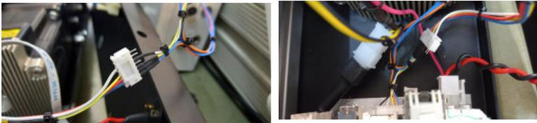
4. Plug power back onto the PCB and the network cable onto the new panel.
