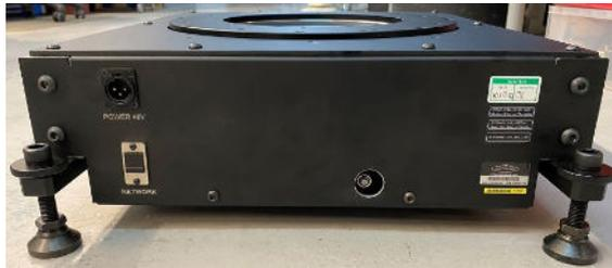
2. Unplug Stepper motor and power from PCB and network from panel.
