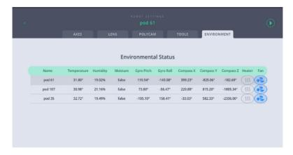
Note that heater can be switched on and remain on when the fan is switched on. Once the fan or heater is turned on, the icon is blue. The heater can remain on for a maximum of 5 minutes, after which it will be switched off automatically.
