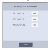
If a selected robot does not go green, then check it is on the same IP address range as the server PC. The Find button does a network wide broadcast, therefore it finds heads even on different subnets.
