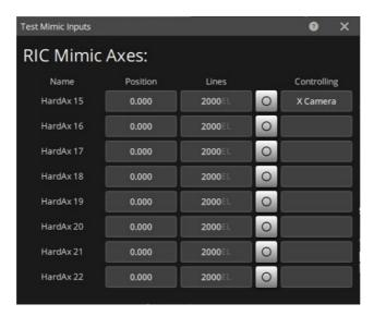
This screen shows the active mimic inputs and the value that is being read from this input port. It show if an axis is assigned to this port. You can also zero the through this screen, but this is not recommended on a live axis.
