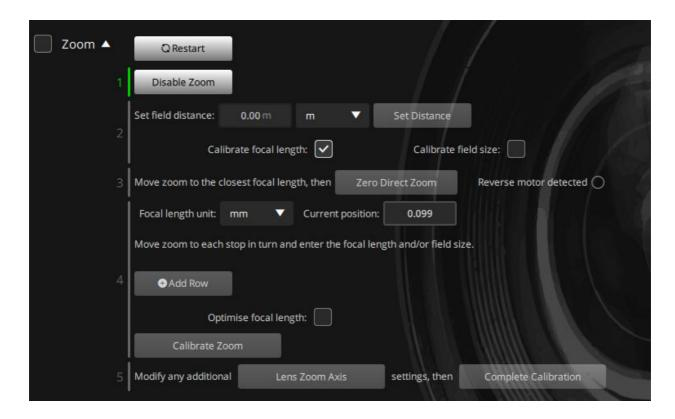
The Zoom Calibration section in the Lens Setup dialog box consists of a series of data entry boxes for the user to enter measurements into that relate to the motion of the zoom axis. The distance measurements are usually done in your selected measure units (for example, centimetres or inches).
