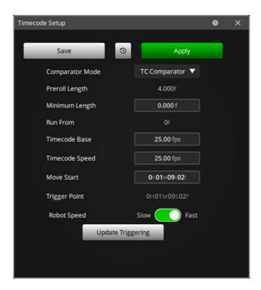
Available on the RT10/12/14 hardware. An OEM timecode comparator is available for use with the older style root boxes, but has limited functionality and cannot generate, only read timecode. (See Serial Devices – TCReader). More details on Timecode Setup covered in Timecode Setup on page 232.
