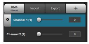
unique address of each device in your DMX setup). In the image, "Channel 1" is the channel name and "[1]" shows the channel number. Hovering over the channel, will show the settings button on the left for the regarding channel.
