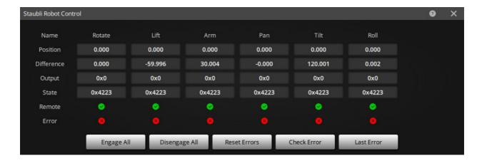
The Staubli status screen shows a listing of each of the Staubli axes along with some status information. Generally speaking the user will not need to look at or use this screen, but information in it may be useful in the case of control issues with the robot.
