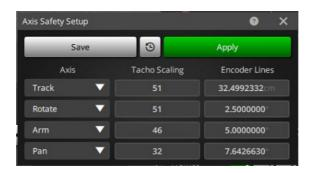
**Axis:** The axis to be monitored. "Not Installed" if no axis is attached to that safety port. Usually which axis has been connected will be designated by MRMC.
