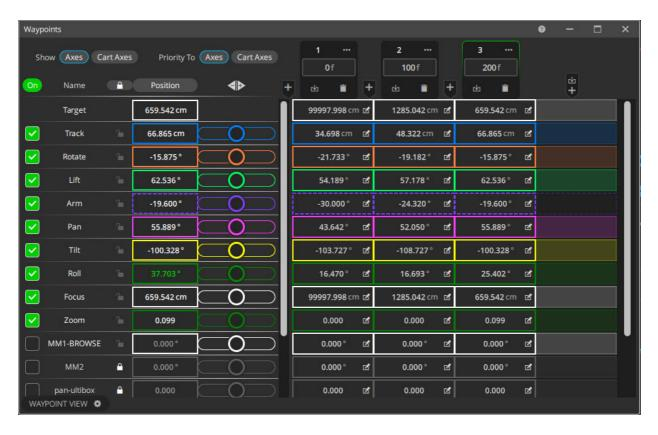
The topmost line is **Positions** which specifies the position number, and is to let you know which position line you are on. If you have more than about five stored waypoints, then they will scroll left and right, and then this line numbering becomes vital. The **Frame count** line is the second line on the Numeric screen, and frame count numbers are entered here by selecting the entry you want to change with the
