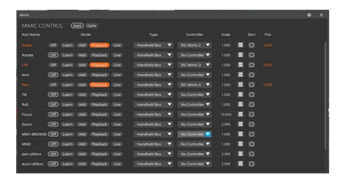
The first five buttons on the display control the state of the axis. Mostly they are off, and as such, no colour is displayed. Any axis that is another mode is show in red so they are easily discernible. Clicking a state puts the axis directly into that state with a single click.
