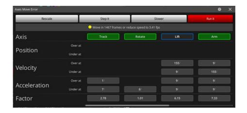
The box that appears will have five buttons on it, a **Rescale** button, which will scale up the move for you, a **Step It** button which will allow you to shoot the move only as a number of stationary exposures, a **Slower** button which will reduce the camera and move speed to a more achievable level and a **Run It** button which will ignore the limits and run the move anyway. You can even close the box to allow you to modify the move as you like using the waypoint view.
