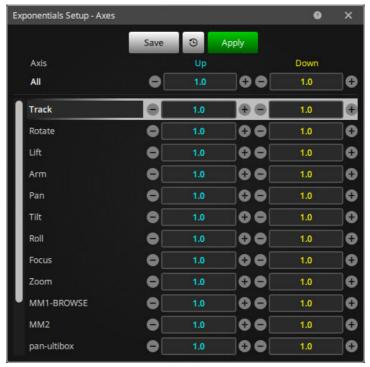
**Up & Down:** In these columns you state the relative proportions of the start and end velocities. For example, if you want the end of the move to be twice as fast as the start, you can enter 1.0 in the start, and 2.0 in the end. This is in fact identical in effect to typing 0.5 in the start and 1.0 in the end. Negative values are not accepted. Exponentials are turned off by entering numbers with a ratio of 1.0 to 1.0 in the start and end columns.
