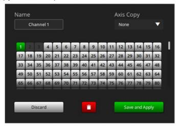
In the right part of the setup window, a + button can be seen. Using that you can add different frame numbers along with your move to add channel value which will adjust the DMX channel.
