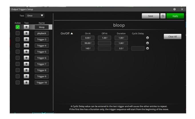
There is an additional way to use the triggers to produce a repeating series. Program in the repeating series you want as an on and off time, leave the next On At blank, but program into the off time at what frame count you want the series to repeat. A series of numbers: on 1.0, off 2.0 followed by a blank on, and then 3.0 in the off column would cause a trigger to turn on and off for one out of every three frames. This is called a Cyclic Trigger.
