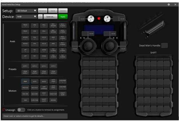
When the Device is selected as HHB for the first time, the default setup appears. The buttons on the hand held box are assigned some default function. On the left
