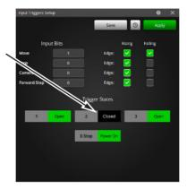
The corresponding numbered **Input Trigger State** in the pop-up should change from **Open** to **Closed**.
