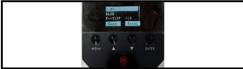
6. Select the same Channel number as that on the motor and press the **ENTER** button.
