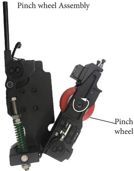
2. Using the same allen key push in the screw cavity to release the pin securing the pinch wheel.
