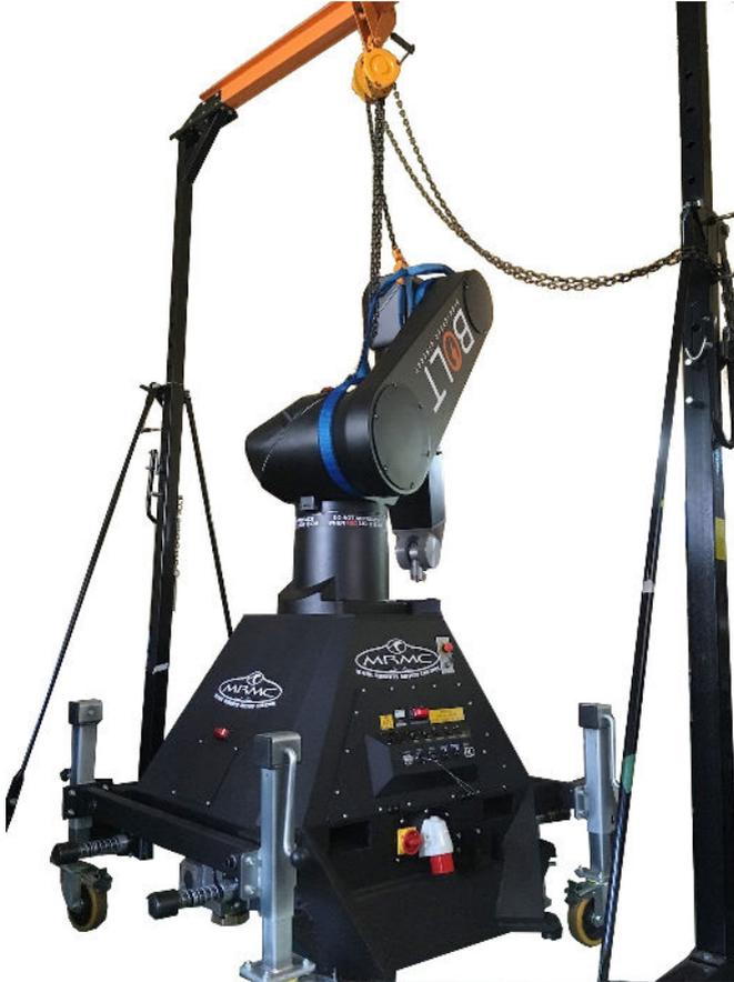
3. Using a 14mm Hex key and 24mm Socket unscrew the 4 x M16 x 60 screws to remove the Bolt arm from the base.
