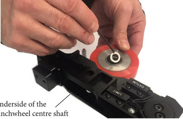
4. Replace the washer on the new pinch wheel carefully and inserting it lined with the screw cavities in the centre shaft of the pinch wheel assembly. Ensure that the washer is inserted towards the underside of the shaft and not on the top.
